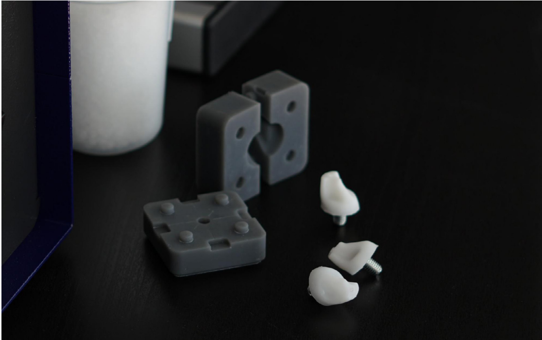
POM football cleats injected in the Holipress from molds printed with Grey Pro Resin.
