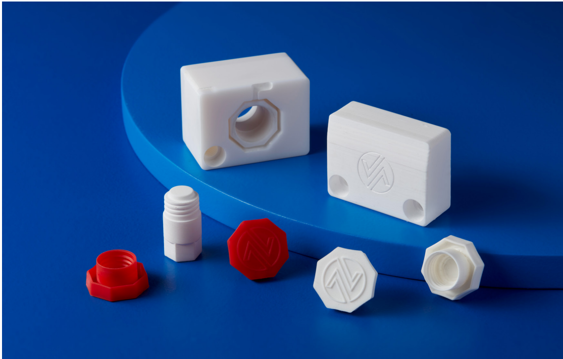
The printed three-parts mold with the caps injected in polyethylene.
