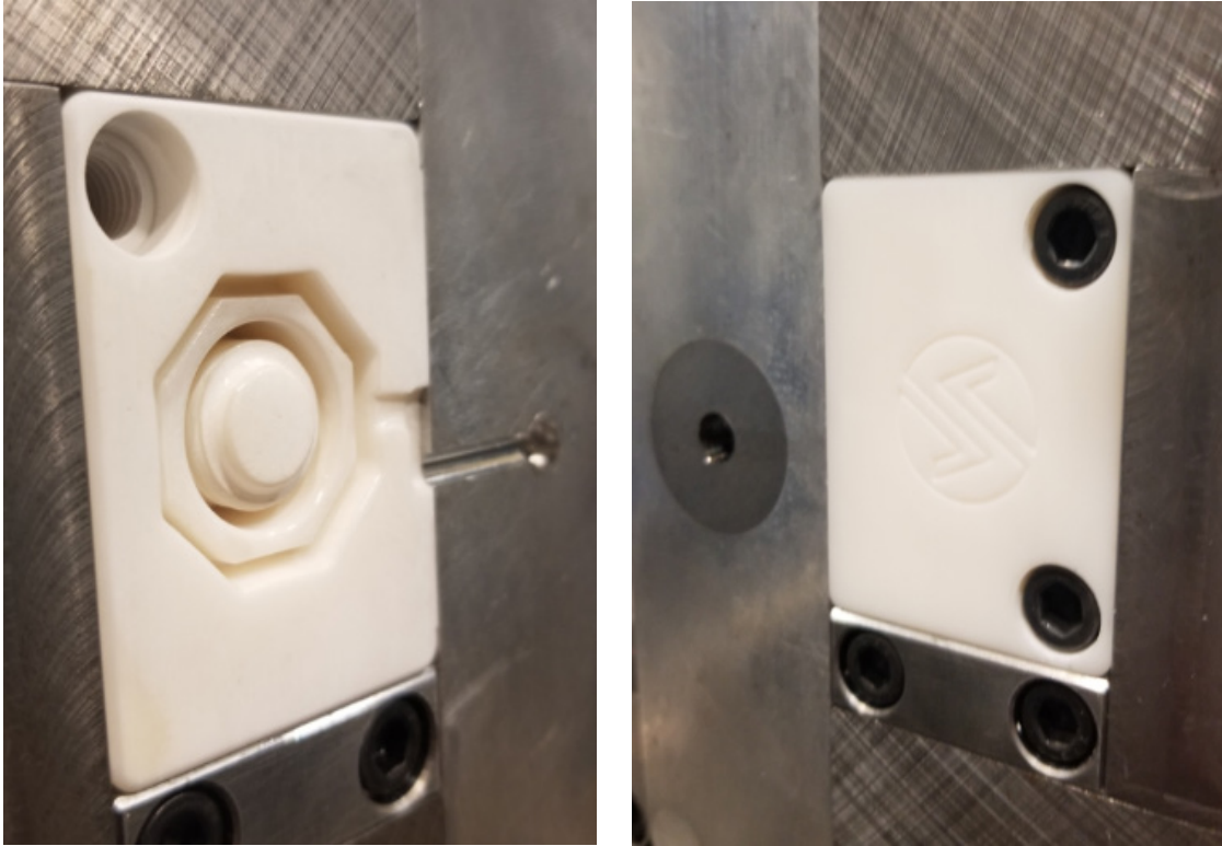
The printed molds were placed into a metallic frame before injection. The side-action core went inside the B side (left) which got locked to the stationary A side (right).
